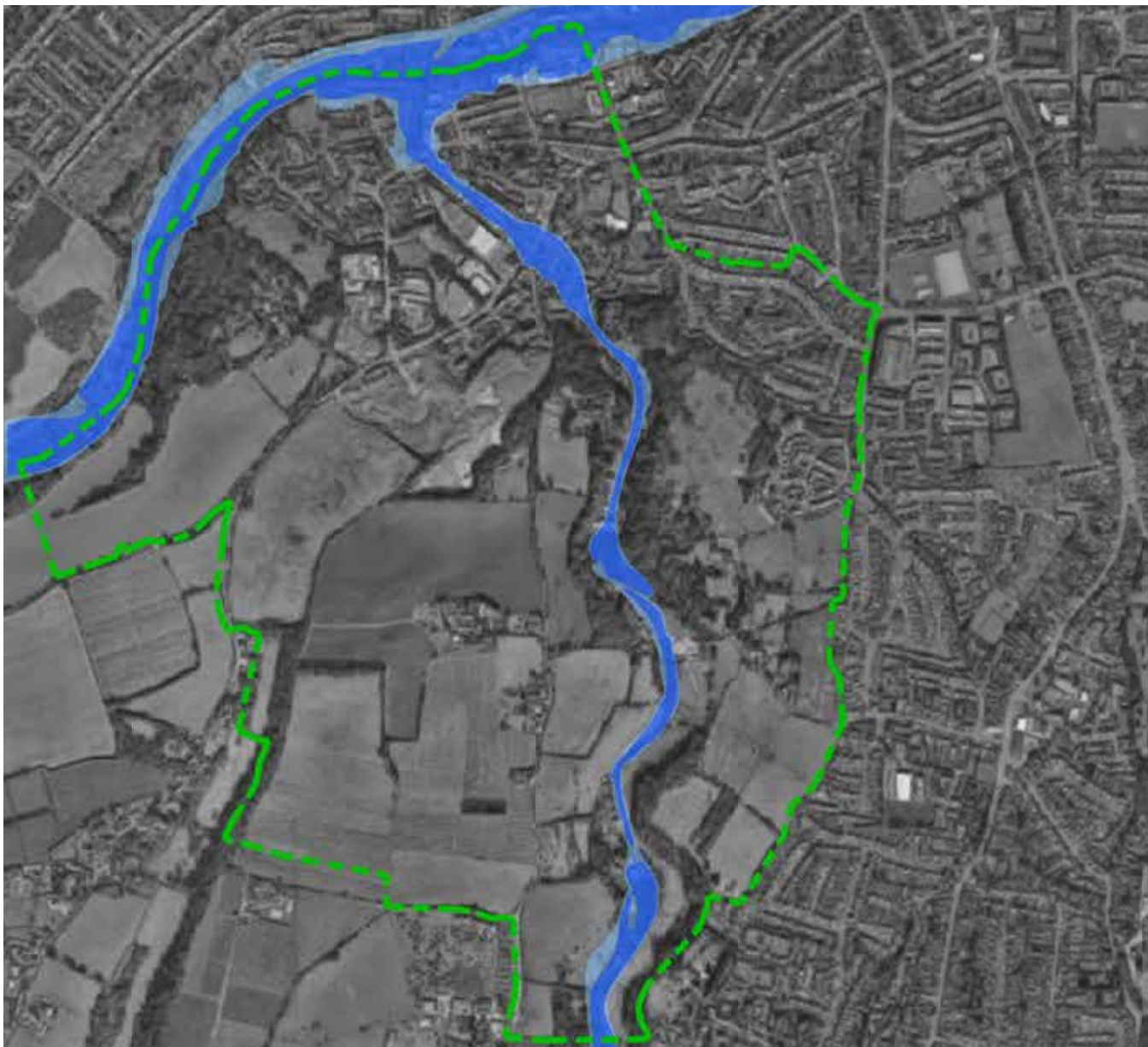
Figure 1.4 (above): Extract from Environment Agency Flood Risk Plan showing Tovil Parish, the steep sides of the valleys are reflected in the limited flood zone area.
